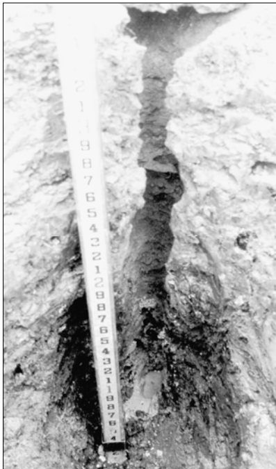
Figure 9. Possible piping macropore exposed in a gully at Rock Run pile (left) resembled piping seen later at Flint Pile Run (right).
