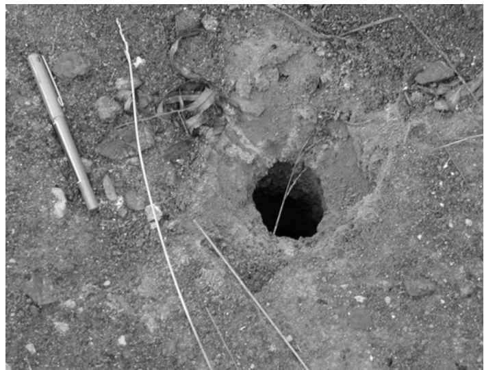
Figure 9. Possible piping macropore exposed in a gully at Rock Run pile (left) resembled piping seen later at Flint Pile Run (right).
