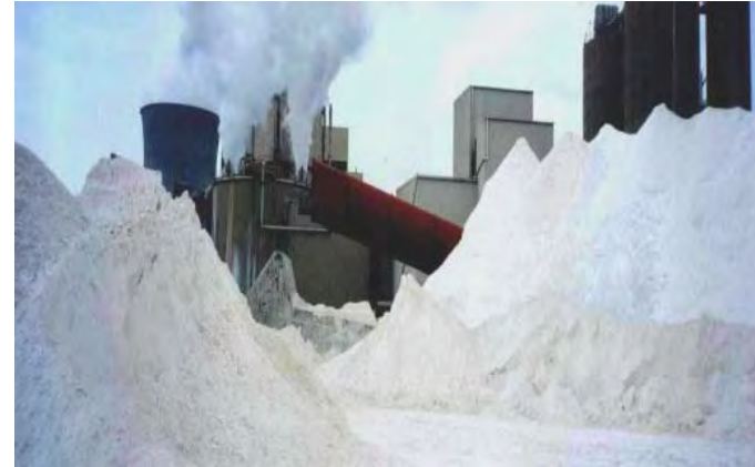
FGD solids ready for disposal
